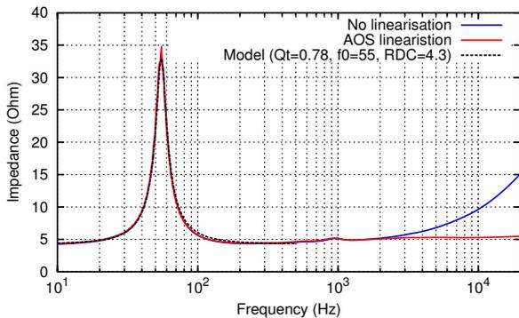
Figure 3: Impedance curves of the two 15W9531G01 midwoofers (parallel) in the box (raw and with linearisation network as designed by AOS). The model curve reflects the impedance of the low-frequency equivalent network of the midwoofers in the closed boxes.
