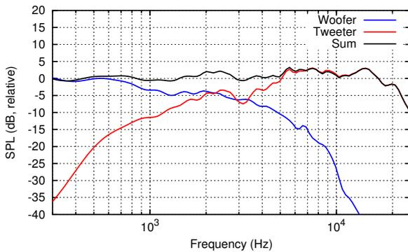
**Figure 7:** Anechoic frequency response with original AOS crossover network (woofers, tweeter, and sum; measured at 1 m distance from the front baffle, on the tweeter axis)
