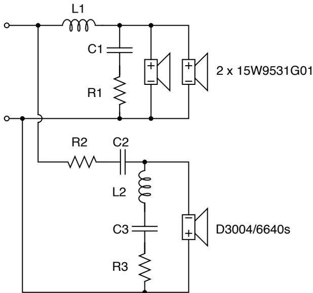
Figure 2: Passive crossover network designed by AOS
