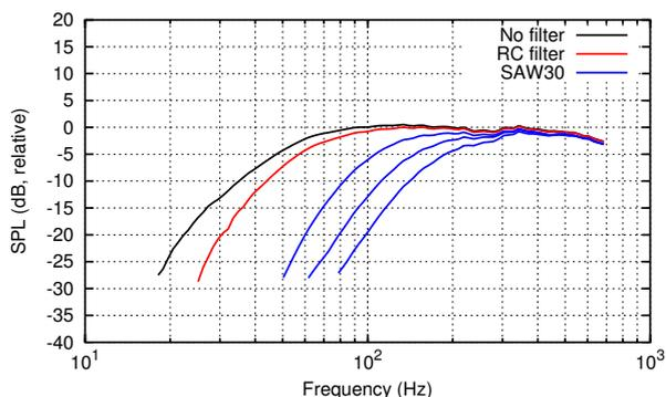
**Figure 16:** S24 bass frequency response measured in the nearfield to gate out room echoes (without filter; RC filter at input of power amplifier, see text; THEL SAW30 set to cut-off frequencies 95 Hz, 132 Hz, 165 Hz)
