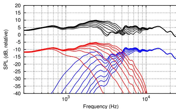
**Figure 13:** Anechoic frequency response of the S24 midwoofers (red), tweeter (blue) and sum (black) with the THEL SAW30 active crossover filter at different crossover-frequency settings ( $f_c = 1419$  Hz, 1975 Hz, 2482 Hz, 3039 Hz, 3611 Hz, 4167 Hz, 4675 Hz, and 5231 Hz)
