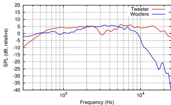
Figure 5: Anechoic frequency responses of tweeter and midwoofers mounted in box, without filters
