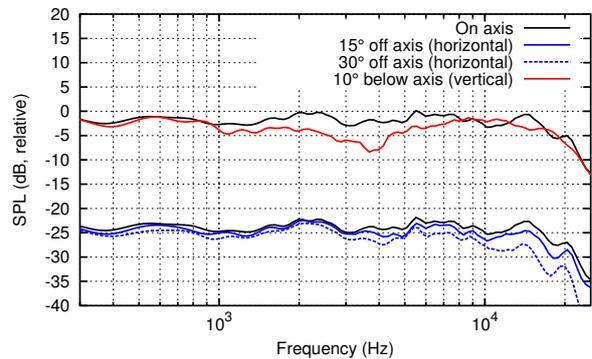
**Figure 9:** Anechoic frequency response at different angles relative to the tweeter axis (measured at 1 m distance from the front baffle)
