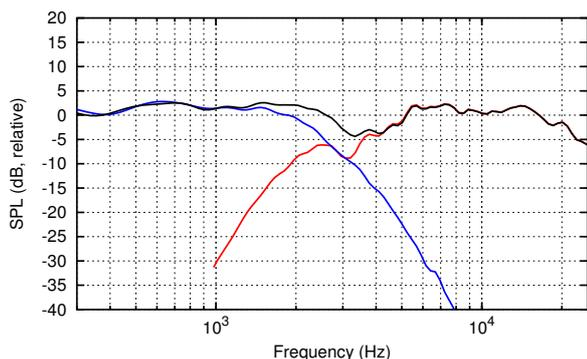
**Figure 14:** Anechoic frequency response of the S24 midwoofers (red), tweeter (blue) and sum (black) with the THEL SAW30 active crossover filter with switches 1, 2 and 4 set to 2482 Hz, and switch 3 set to 1975 Hz. The baffle step compensation was set to 12 h with  $C = 33$  nF.
