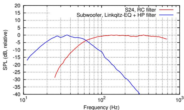
**Figure 17:** Bass frequency responses of the S24 and the subwoofer, measured in the nearfield to gate out room echoes (S24 with RC high-pass filter, subwoofer with 18 dB/octave low-pass filter and Linkwitz pole-zero equalisation)
