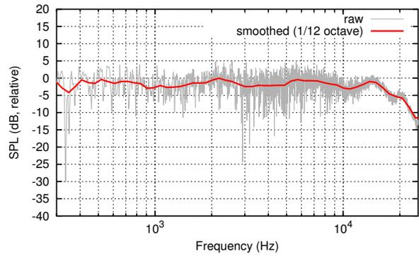
**Figure 8:** In-room frequency response (calculated using the first 200 ms of the impulse response, measured at 1 m distance from the front baffle on the tweeter axis)
