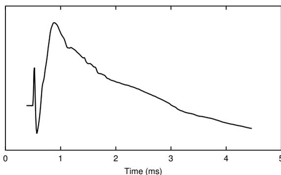
**Figure 15:** Step response of the S24 with the THEL SAW30 active crossover filter with switches set as in Fig. 14.
