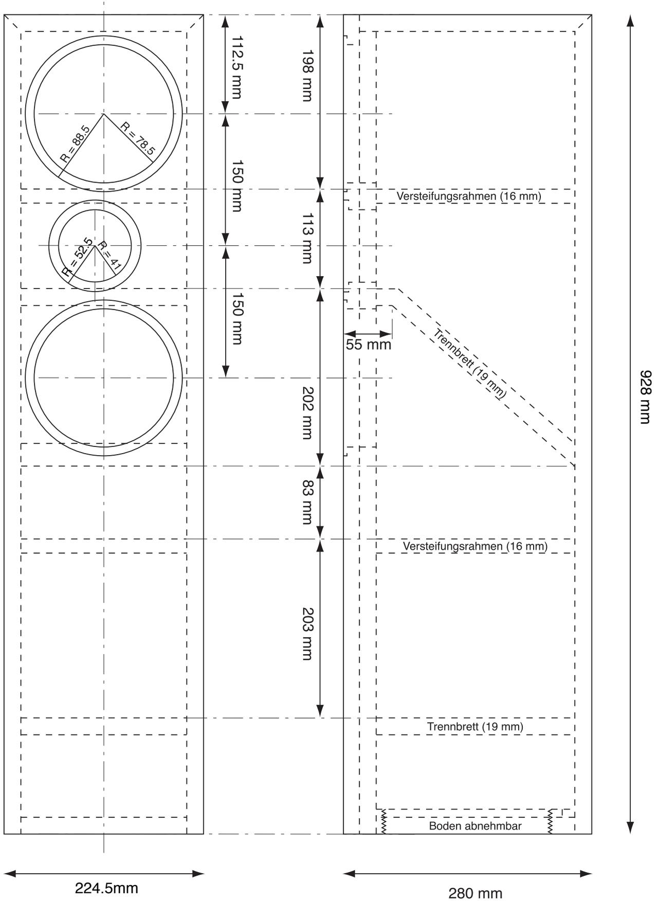
Figure 1: Enclosure drawing of my S24. The midwoofer offset relative to the front baffle is not shown.
