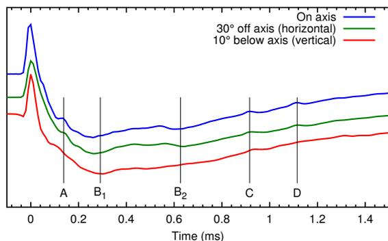
**Figure 10:** Step response at different angles relative to the tweeter axis (measured at 1 m distance from the front baffle). A: echo of the tweeter sound wave reflected at the aluminium rings. B1–B2: superposition of echoes reflected at the baffle edges and the aluminium rings. I don't know the origin of echoes C and D.
