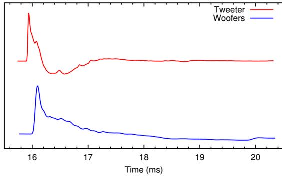
**Figure 6:** Step responses of tweeter and midwoofers mounted in box, without filters
