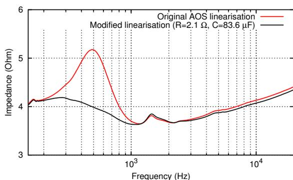
**Figure 11:** Impedance curves of the D3004/664000 tweeter with original AOS linearisation network and modified network
