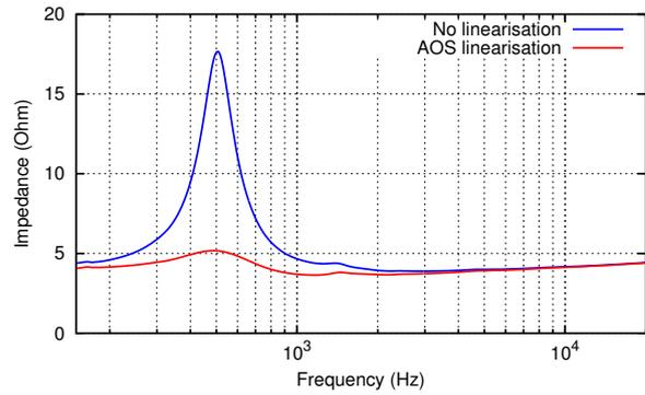
Figure 4: Impedance curves of the D3004/664000 tweeter (raw and with linearisation network as designed by AOS)
