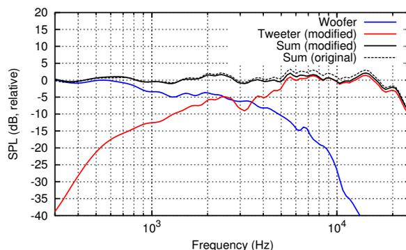
**Figure 12:** Anechoic frequency response with modified tweeter filter network (red) in comparison to the original AOS filter. The midwoofer filter is identical to the original AOS filter.
